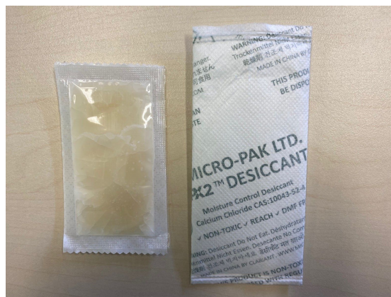
Fig. 2 Calcium chloride packaging consists of an inner plastic pouch and an outer non-woven layer
