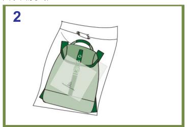
At time of final packing, two pieces of 25cm x 25cm Micro-Pak® Sheet should be placed flat inside the polybag on both sides of the backpack. Do not fold or crumple the sheet.
