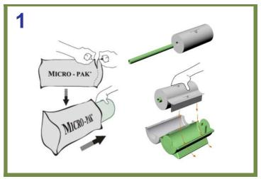
Open Micro-Pak® Sheet foil pouch. Remove roll of Micro-Pak® PE Sheets, fit into the roller and place in the Micro-Pak® Sheet dispenser box.
