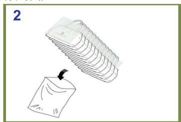
At time of final packing, several pieces of 25cm x 25cm Micro-Pak® Sheet should be used with one sheet placed flat between each bag.
