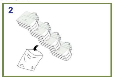
At time of final packing, several pieces of 25cm x 25cm Micro-Pak $\circledR$  Sheet should be used with one sheet placed flat between every two to three bags.
