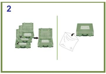
At time of final packing, two continuous pieces of 25cm x 25cm Micro-Pak® Sheet should be placed flat inside each of the nested luggage. Additional two continuous pieces of 25cm x 25cm Micro-Pak® Sheets should be placed flat on top of the outer luggage and put inside the polybag. Do not fold or crumple the sheet.
