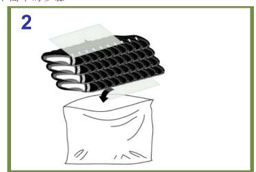
At time of final packing, two pieces of 60cm x 40cm Micro-Pak® Sheet should be placed inside the polybag together with the shoes.
