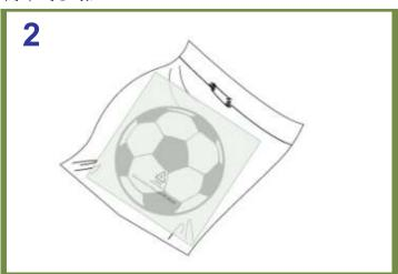
At time of final packing, one piece of 25cm x 25cm Micro-Pak® Sheet should be placed flat inside the polybag together with the football / soccer ball.
