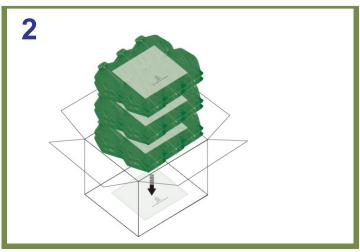
At time of final packing, one piece of 40cm x 30cm Micro-Pak® PE Sheet should be placed flat every two layers of the products. One piece at the bottom of the box, one piece between 2nd and 3rd layer, one piece between 4th and 5th layer AND one piece on the top layer of the products.
