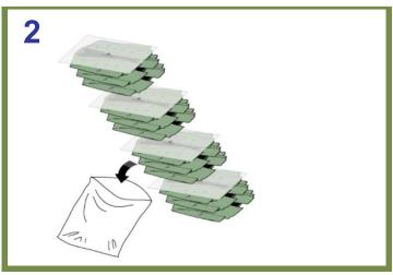
At time of final packing, several pieces of 60cm x 40cm or two continuous 40cm x 30cm Micro-Pak® Sheet should be used with one sheet placed flat between every two to three jackets. Do not fold or crumple the sheet.
