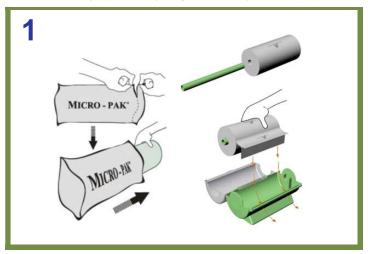
Open Micro-Pak® Sheet foil pouch. Remove roll of Micro-Pak® PE Sheets, fit into the roller and place in the Micro-Pak® Sheet dispenser box.
