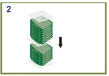
At time of final packing, three pieces of 25cm x 25cm Micro-Pak® Sheet should be placed flat at the bottom, in the middle and on top of each section of products and put inside the master polybag.
