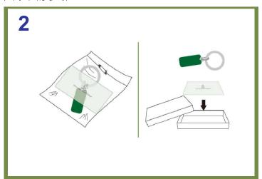
At time of final packing, one piece of 16cm x 8cm Micro-Pak® Sheet should be placed inside the polybag or box together with the product.
